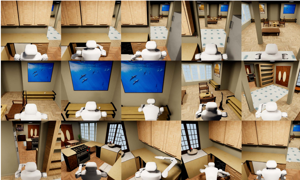
Figure A.6: Successful task completion by a participant. The robot navigates to a dishwasher and opens it, moves to a table to collect teacups, returns to the dishwasher, places the teacups inside, and closes it.
