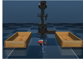
Figure 5: Setup for the Multi-Stage Manipulation with Scripted Data tasks consist of a simulated WidowX arm with 2 identical bins. In the center of the scene are two objects that are categorized as shoes or toys which the agent has to sort into their respective bins.
